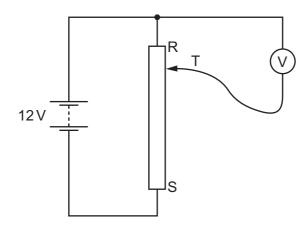
As the sliding terminal T is moved from R to S, what happens to the reading on the voltmeter?
